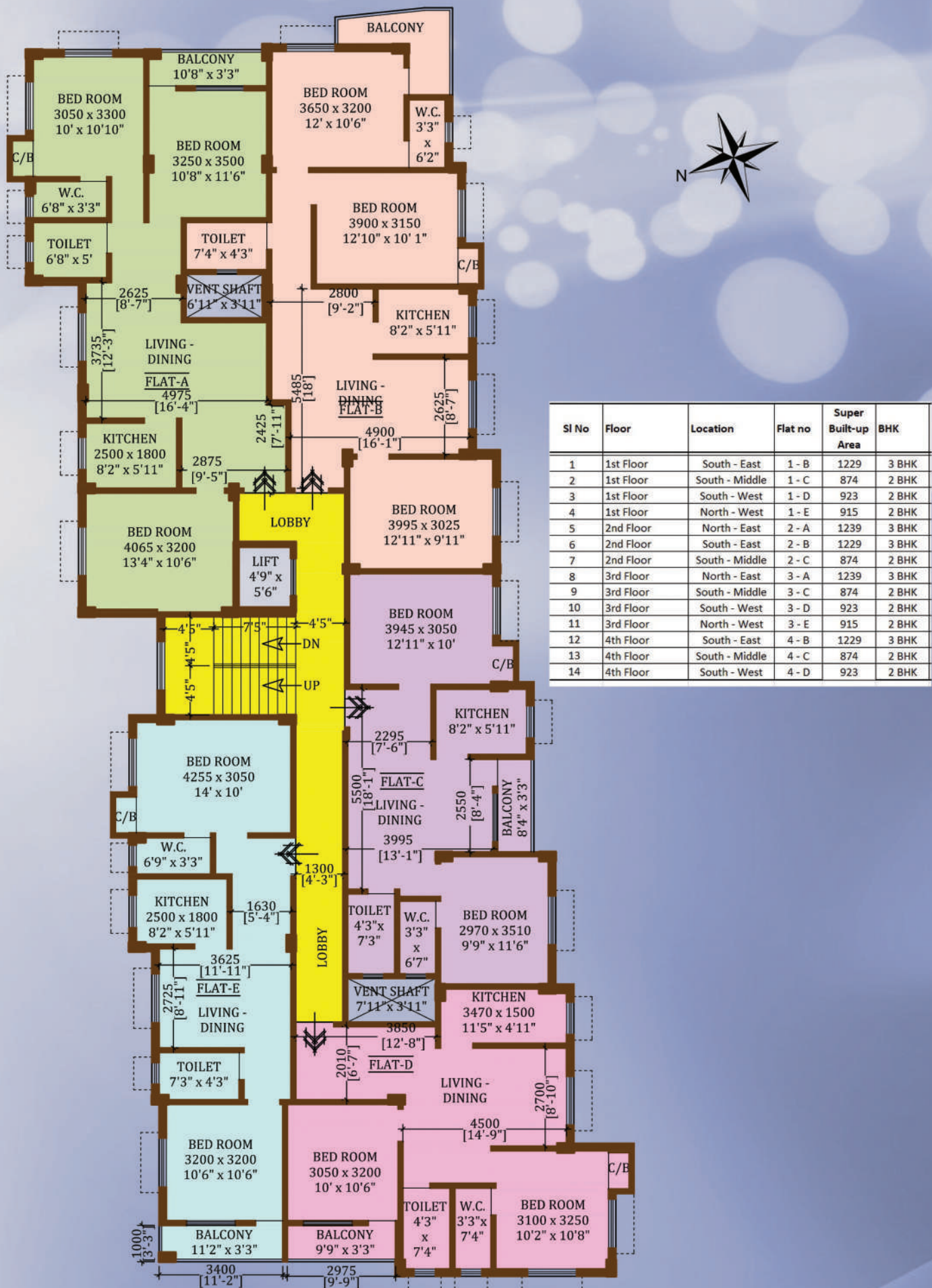
PROPOSED TYPICAL (1ST, 2ND, 3RD & 4TH) FLOOR PLAN
